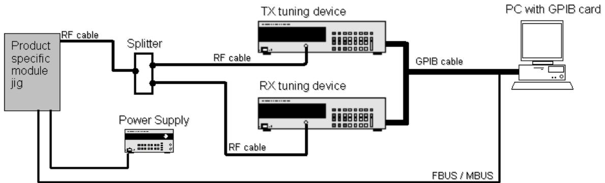
GPIB addresses are not defined. Component finds the addresses and uses them automatically. If several TX tuning devices are connected, this component uses Agilent (VSA or PSA). In RX side, Agilent has highest priority.
