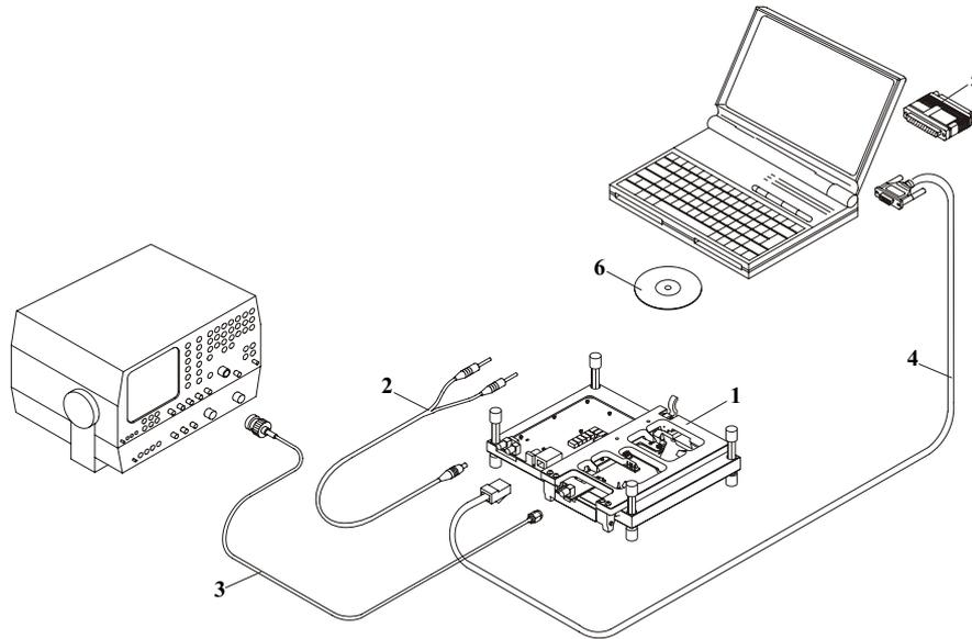
**Figure 3:Module jig concept**
