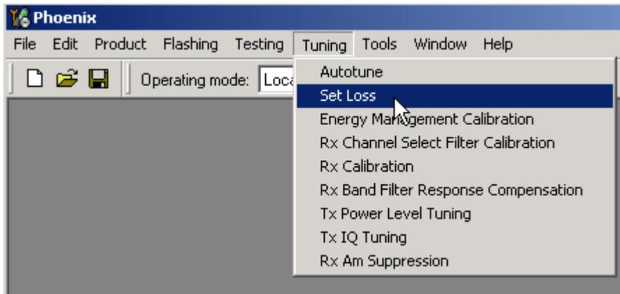
This is the component for saving RF-losses (of cables and jigs) to file. These loss values are needed when you tune the phone with Phoenix (using Auto-Tune component). When you measure the losses you have to be very careful, because these values affect directly how well the phone is tuned.
