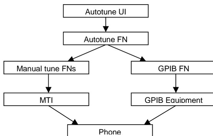
Autotune is a pair of two different components. One is User Interface and the other is Functional. UI does not contain any functionality. MTI takes care of phonet messages.
